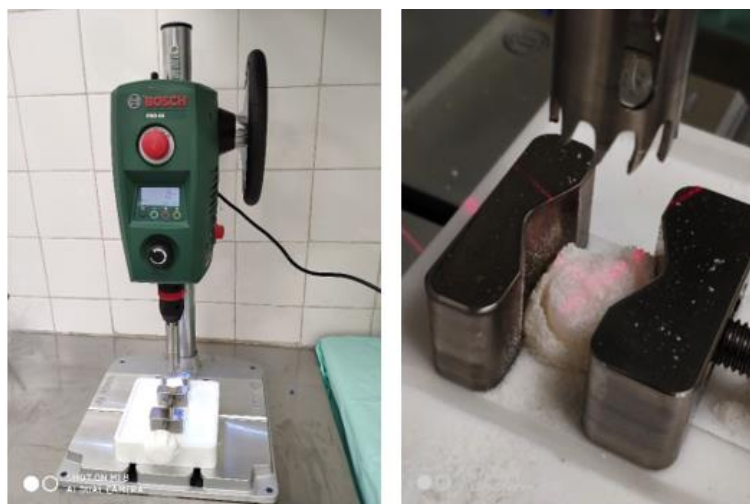
Figure 2: Equipment which uses laser for the correct placement and cutting of the bone piece
